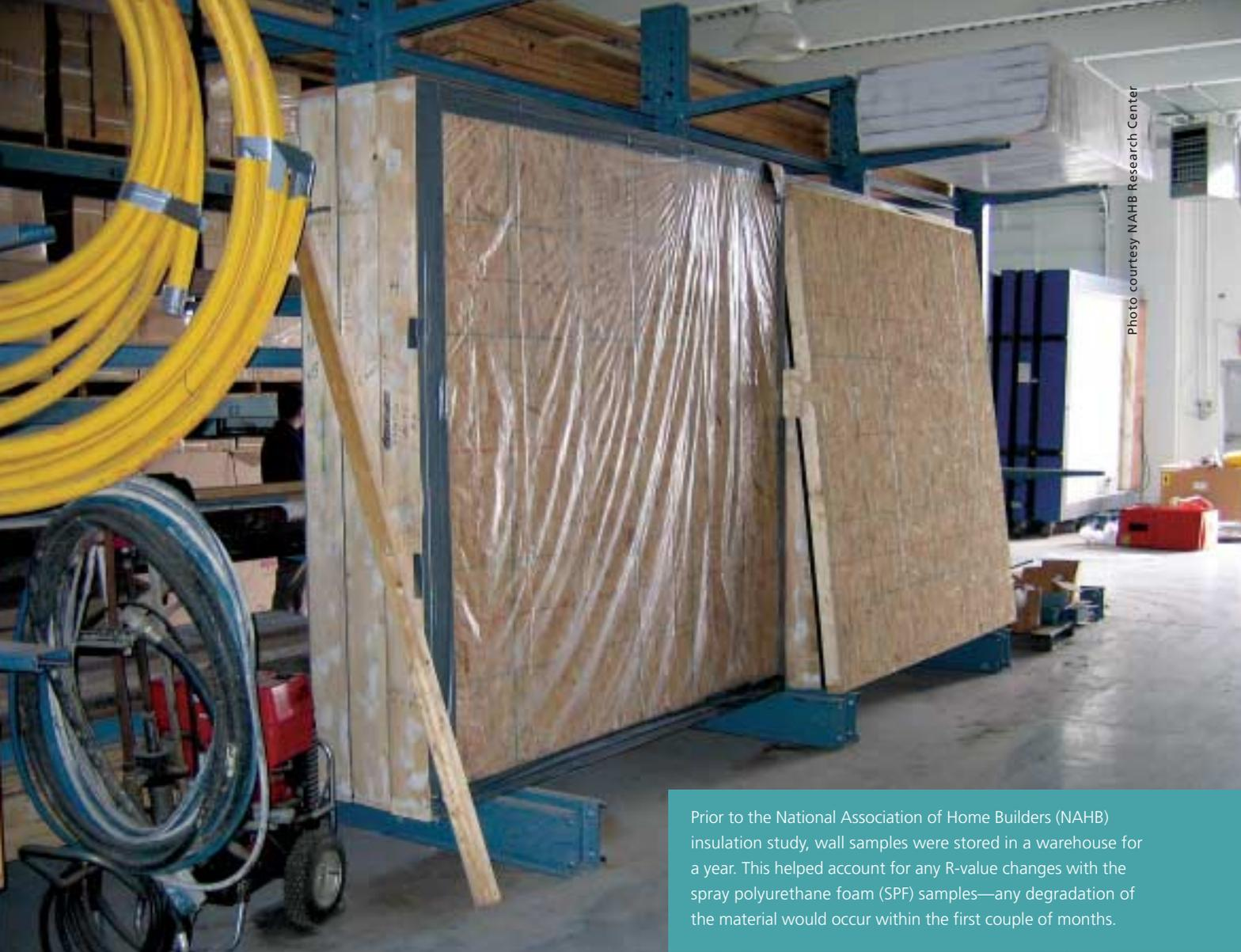
Prior to the National Association of Home Builders (NAHB) insulation study, wall samples were stored in a warehouse for a year. This helped account for any R-value changes with the spray polyurethane foam (SPF) samples—any degradation of the material would occur within the first couple of months.
